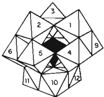
Figure 1. Coordination polyhedral representation of the Keggin polyoxometalate polyanion \text{PW}_{12}\text{O}_{40}^{3-} ( =(\text{PO}_4)^{3-}(\text{W}_3\text{O}_9)_4^0 ) showing the central \text{PO}_4^{3-} tetrahedron in black and the four \text{W}_3\text{O}_9 triads composed of edge-sharing \text{WO}_6 octahedra. The \text{PW}_{12-x}\text{V}_x\text{O}_{40}^{3-x} derivatives are formed by replacement of the indicated W (e.g. in 1,2- \text{PW}_{10}\text{V}_2\text{O}_{40}^{5-} the 1-W and 2-W) by V.
